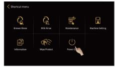
Step 3: Operate according to the prompts on the coffee machine interface, and enter the soft-off state after the shutdown is completed. (In soft-off state, press and hold the circular button for 3 seconds to restart the coffee machine.
